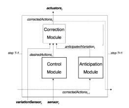
Fig. 1. Overview of the control architecture
