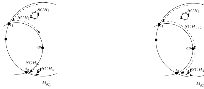
Figure 13 Building faces using union-find. SCH_1, SCH_2, SCH_3, SCH_4 define the same face. At i_1 and i_2 , we start two new faces with SCH_1 and SCH_2 . Before the meridian reaches ep , two faces are defined, both with two SCH. After ep , one face with three SCH remains. This merge is achieved using union-find.
