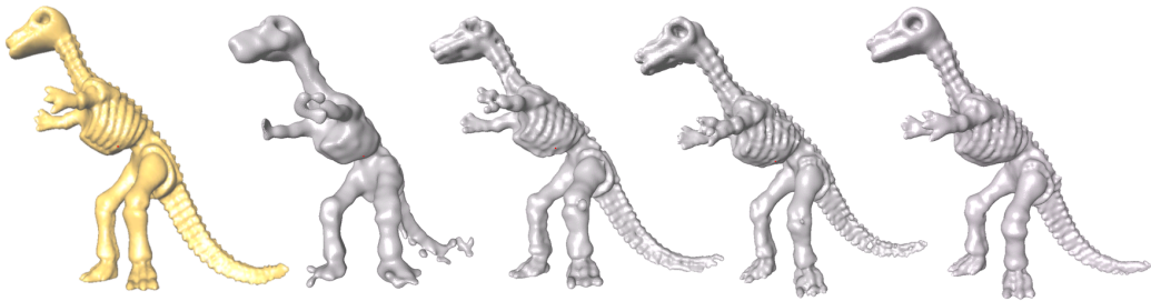
Figure 9: Reconstruction sequence of the Dinosaur with increasing number of centers. From left to right: original, then reconstruction with 1K, 3K, 4K and 5K centers.
