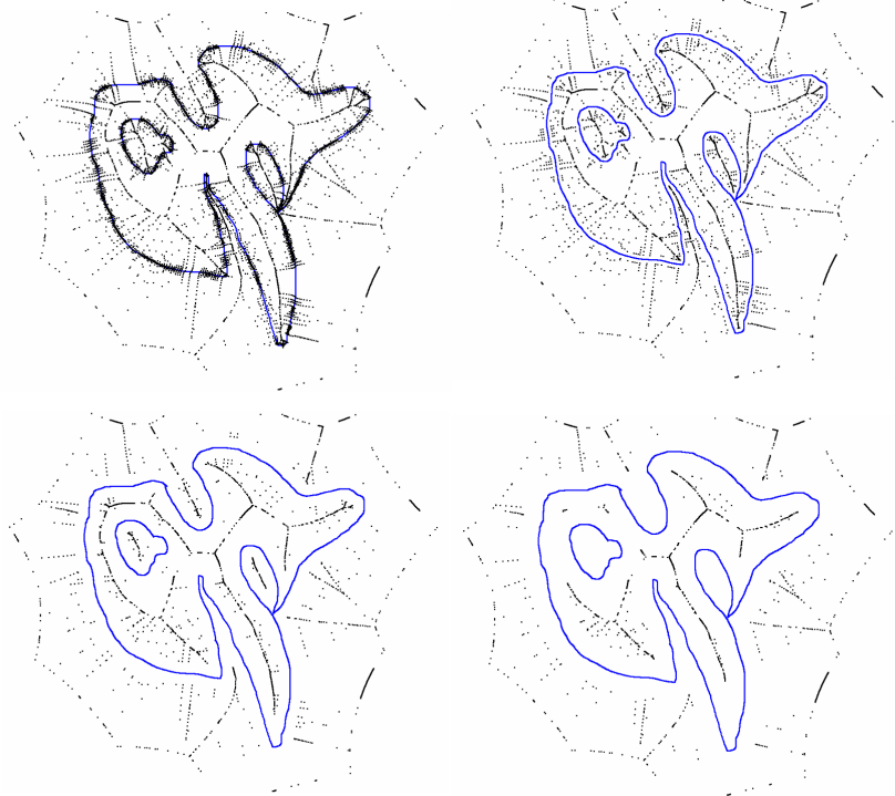
Figure 2: Medial axis filtering on a 2D shape (blue). The \lambda -medial axis is depicted in black. Top left: all extracted poles. Top right: pole filtering with parameter \lambda = 0.01 . Bottom left: \lambda = 0.03 . Bottom right: \lambda = 0.05 . To get a better sense of these parameters: the diagonal length of the bounding box of the input point set is 1.4.
