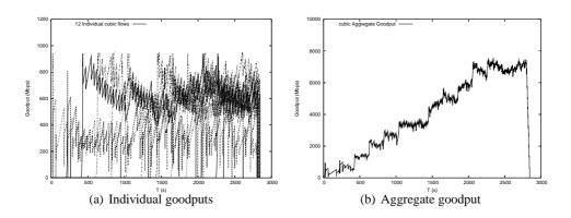
Figure 12: CUBIC in AIST-GtrcNET-10 with 100 ms RTT
