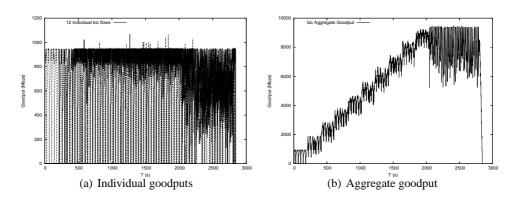
Figure 11: BIC in AIST-GtrcNET-10 with 100 ms RTT
