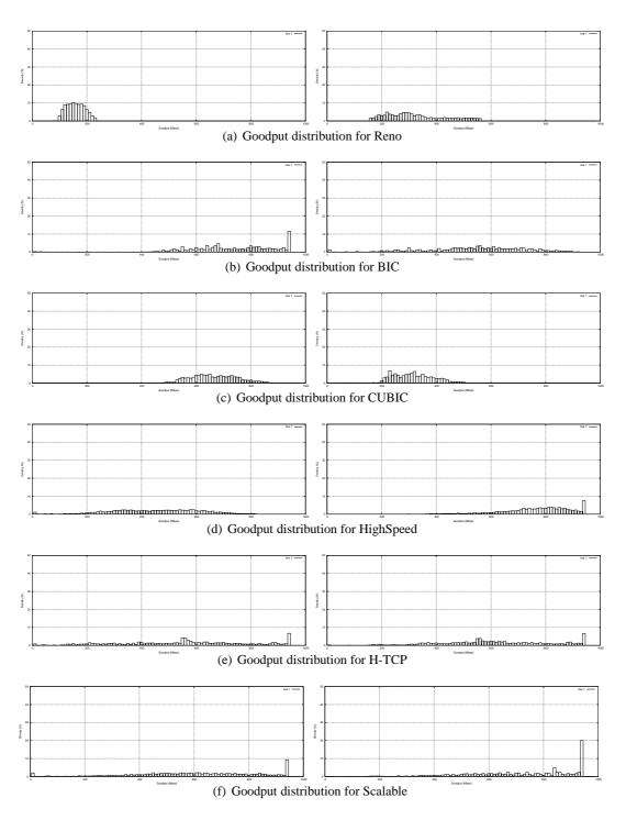
Figure 21: Examples of Goodput distribution for 100 ms RTT when 12 nodes are active, in AIST-GtrcNET-10 ms
