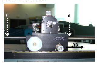
Figure 2. Cart as the controlled system
