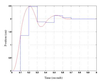
Figure 5. Response time to the reference under (1,10)-firm constraint ( $\{10000000000\}$ )
