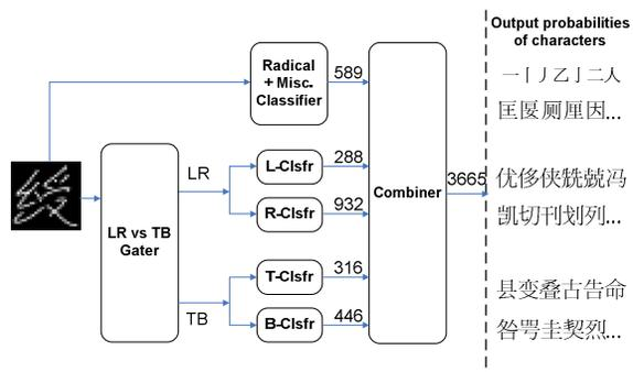
Figure 8. The example recognizer with a gater.
