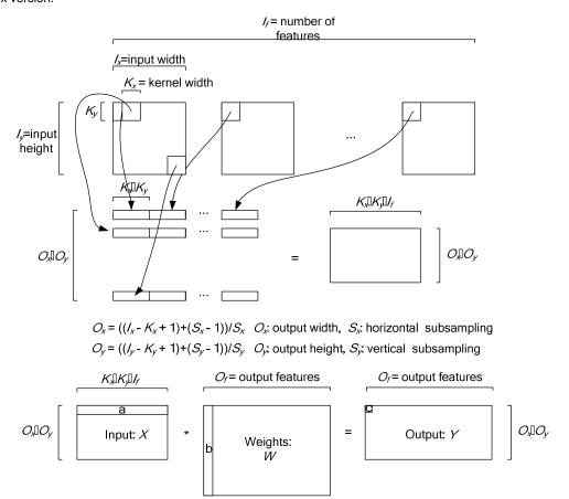
Figure 3. Unrolling the convolution operations in a convolutional layer (biases, sub-sampling, and non-linearity omitted), to produce a matrix-matrix product version.
