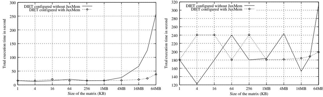
Figure 4: Total execution time ( $t$ ) of a test with one persistent matrix of variable size when DIET is configured with and without JUXMEM. The execution time of the service is  $s$  ( $s = 5$  seconds on the left and  $s = 60$  seconds on the right).
