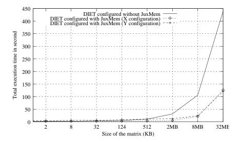
Figure 5: Total execution time (t) of the DGEMM test when DIET is configured with and without JUXMEM (using two different configurations of JUXMEM X and Y).
