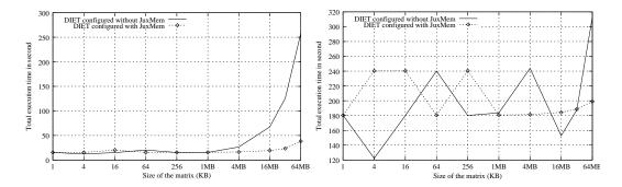
Figure 4: Total execution time (t) of a test with one persitent matrix of variable size when DIET is configured with and without JUXMEM. The execution time of the service is s (s = 5 seconds on the left and s = 60 seconds on the right).
