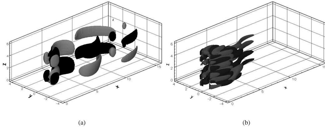
Figure 5: (a) Streamwise vorticity in the wake obtained at  $Re = 200$  and  $t = 92.4$ . The gray surface corresponds to  $\omega_x = 0.1$ , while the black one to  $\omega_x = -0.1$ . (b) Streamwise vorticity in the wake obtained at  $Re = 300$  and  $t \simeq 35$ . The gray surface and black surfaces correspond to  $\omega_x = 0.05$  and  $\omega_x = -0.05$  respectively.
