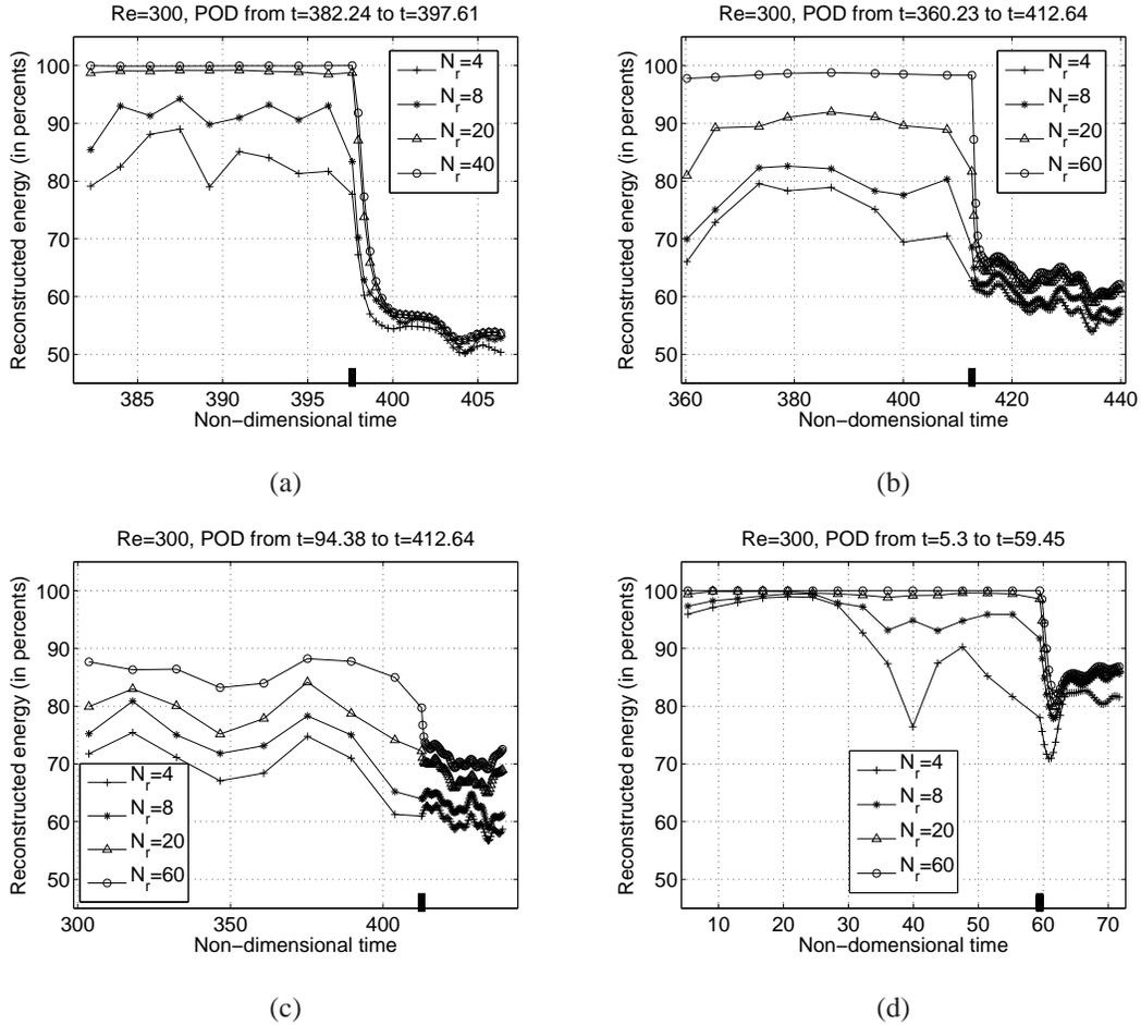
Figure 8: Percentage of reconstructed fluctuating energy for flow fields inside and outside the database.  $N_r$  is the number of modes. (a) POD1, (b) POD2, (c) POD3 and (d) POD4. The mark on the abscissa denotes the limit after which the reconstructed snapshots do not belong to the database.
