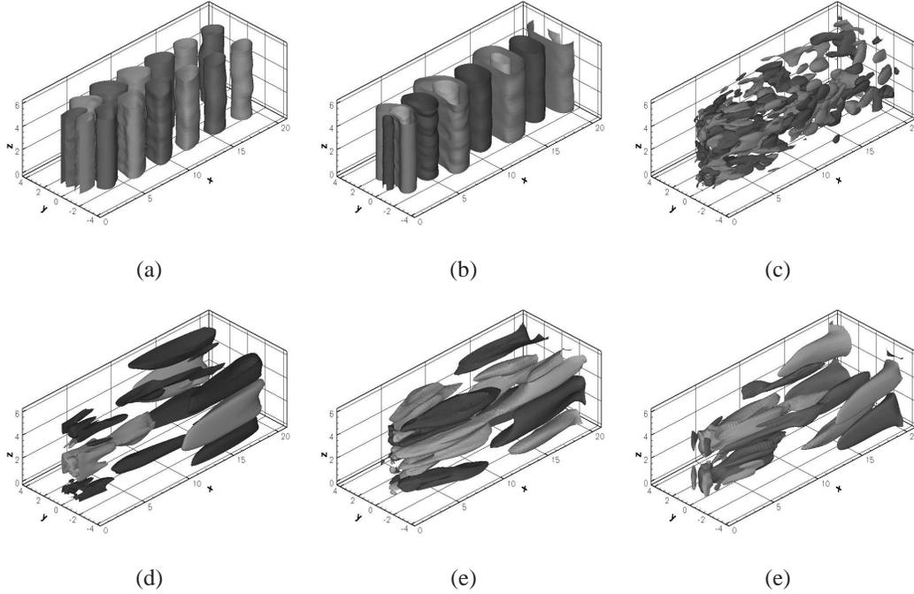
Figure 9: Components of the first (top) and third (bottom) mode relative to POD3. (a)  $x$ -component: light gray 0.015, dark gray -0.015; (b)  $y$ -component: light gray 0.05, gray 0.01, dark gray -0.04; (c)  $z$ -component: light gray 0.0035, dark gray = -0.0035; (d)  $x$ -component: light gray 0.032, dark gray -0.032; (e)  $y$ -component: light gray 0.02, dark gray -0.02; (f)  $z$ -component: light gray 0.025, dark gray -0.025.
