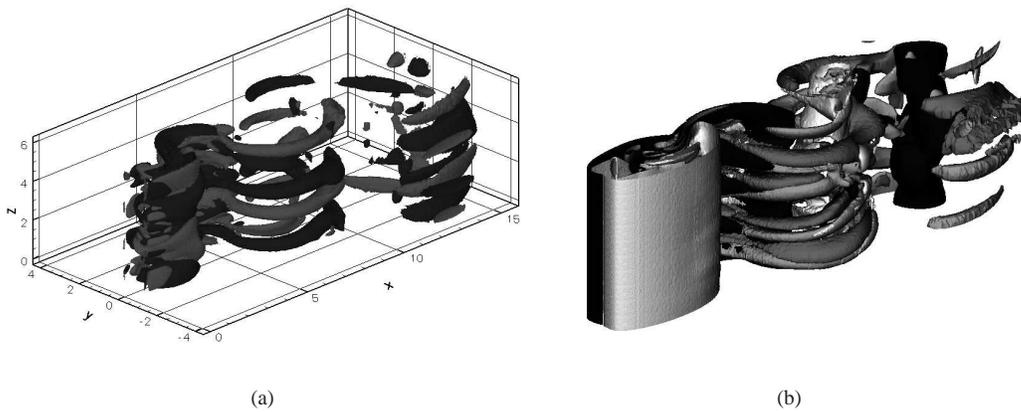
Figure 6: (a) Streamwise vorticity in the wake obtained at  $Re = 300$  and  $t \simeq 57$ . The gray surface identifies  $\omega_x = 0.4$  and the black one  $\omega_x = -0.4$ . (b) Streamwise and spanwise vorticity components in the wake obtained at  $Re = 300$  after the transient. The black and light gray surfaces correspond to  $\omega_z = -0.4$  and  $\omega_z = 0.4$  respectively. The streamwise tubes identify  $\omega_x = 0.4$  and  $\omega_x = -0.4$  respectively.
