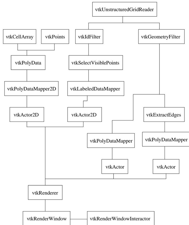
Figure 12: Labeled points visualization pipeline.
