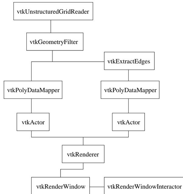
Figure 8: Mesh visualization pipeline.
