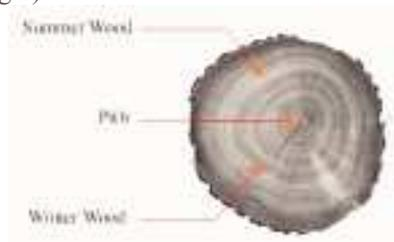
Fig. 1. Radial section of a trunk.
