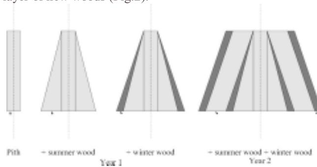
Fig. 2. Secondary growth model of the tree.
