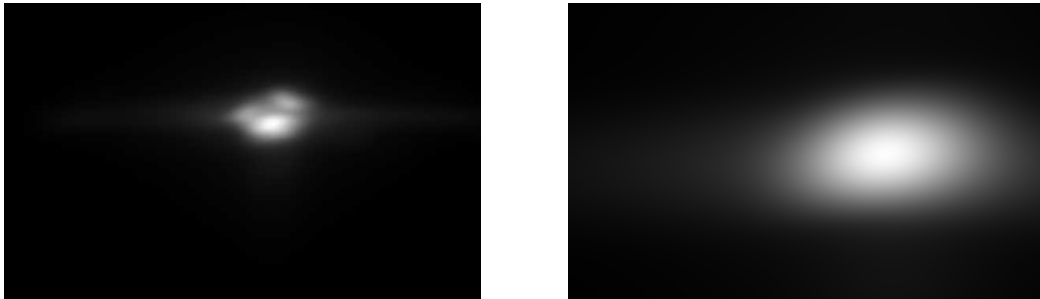
Figure 11: Projection on a wall parallel to the cylinder axis. The intensities have been scaled rescale to [0, 1] in order to show the pattern variation with the distance (near-field effect). Left, distance source plane = 120 cm; right, distance source plane = 300 cm.
