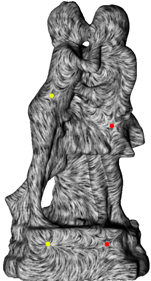
Fig. 10. A vector field defined using our representation on a genus-3 surface. Yellow dots are first-order singularities with indices -1 and 1. Red dots are higher-order singularities of indices both -2.
