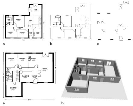
Fig. 18a–c. Symbol recognition for a simple drawing (1700×1600 pixels) vectorized in about 300 segments and arcs. a A drawing. b Thin lines. c Symbols
