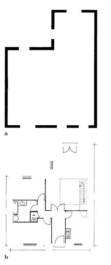
Fig. 5a,b. Thin/thick separation. a Thick lines. b Thin lines
