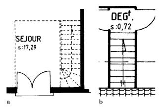
Fig. 14. Staircases in a typical architectural drawing. a First floor. b Second floor
