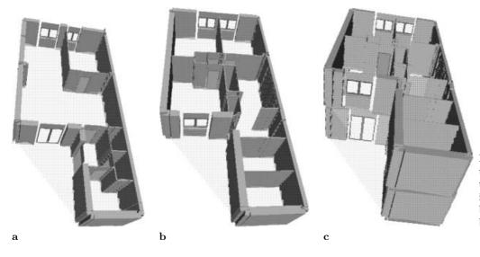
Fig. 20a-c. 3D reconstruction of a private house from the architectural drawings of its floors. a First floor 3D. b Second floor 3D. c Whole building 3D
