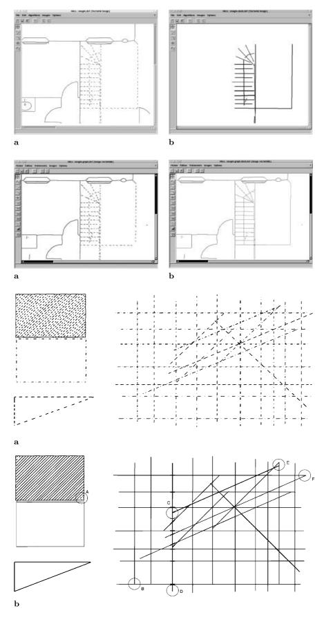
Fig. 11a,b. Dashed lines detection. a Source image. b Detected dashed lines
