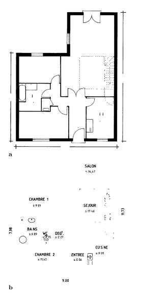
Fig. 3a,b. Text/graphics separation. a Graphics layer. b Text layer
