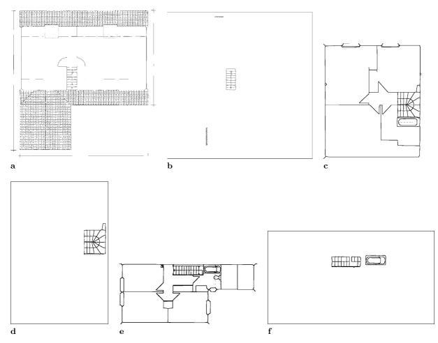
Fig. 16a-f. Vectorized drawings (a, c, e) and recognized staircases (b, d, f)—before user interaction and correction
