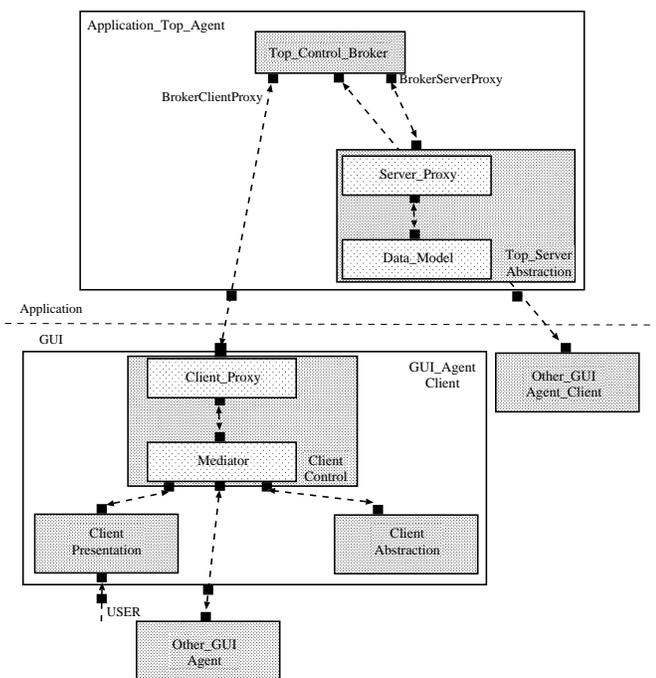
FIG. 4 —. Combination of Broker and PAC Architectural Patterns
