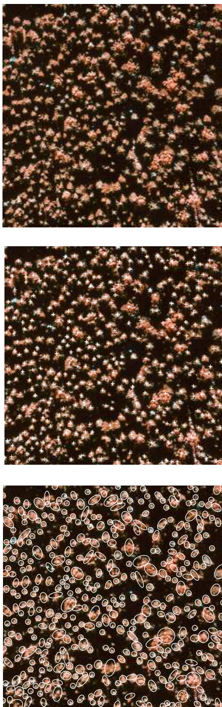
Figure 4: Result on a natural forest (top: initial image © SUAS, middle: detected trees, bottom: tree templates)
