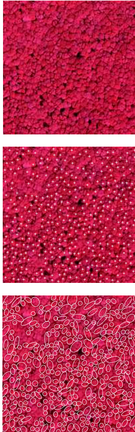
Figure 5.82 Result on a dense oak forest (top: initial image © IFN , middle: detected trees, bottom: tree templates)
