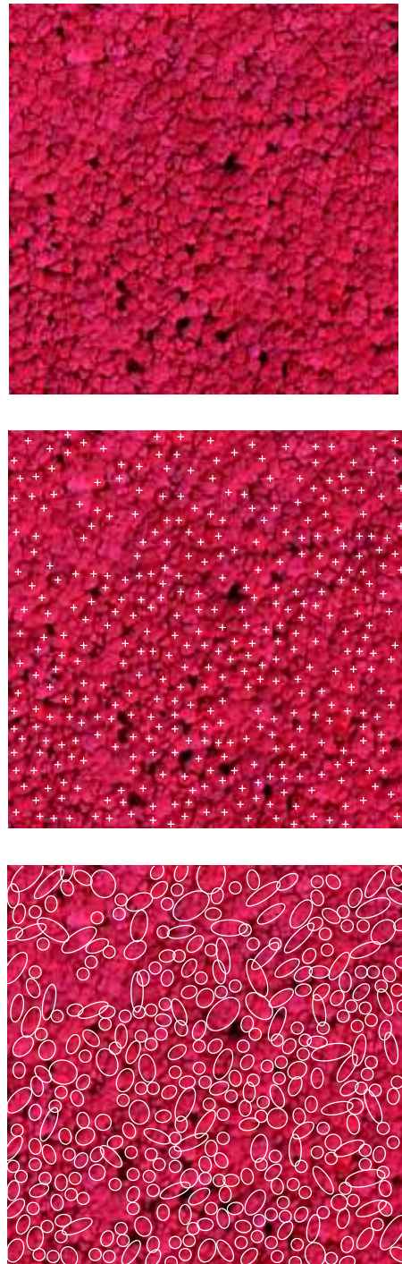
Figure 5.23: Result on a dense oak forest (top: initial image © IFN , middle: detected trees, bottom: tree templates)
