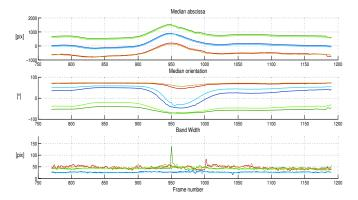
Fig. 2. Evolution of the DVP and the characteristics of the RMs along the Antibes sequence. Top: chronogram of the DVP location in left (red) and right (green) images. Bottom: tracking of the three RMs (red left, blue middle, green right) RMs for the 2-lanes road.
