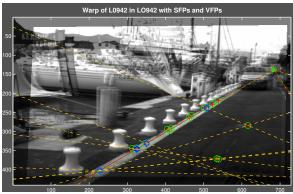
Fig. 5. Comparison between homography computed classically (top) and that extracted from the super-homography (bottom). The current image with green features is warped into the last one with red features. The VFPs (blue '\o') are intersections of pencil of RMs and the virtual (orange dashed) lines.
