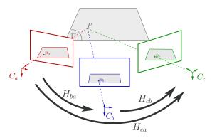
Fig. 1. The projections of the point  ${\bf P}$  are cross-linked thanks to the homographies induced by the  $\pi$  plane in each image.
