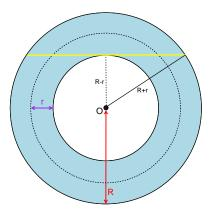
Figure 5: Viewing a torus from top. We show how the longest ray's length (in yellow) can be easily computed from the tokamak's parameteric equation. r is the minor radius and R the major radius of the torus.
