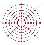
Figure 1: Samples of a typical poloidal plane. Constant radial progression of the meshes for all the rings can be observed, implying oversampling for the rings of low radius.
