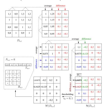
Figure 4: Compression example for a subpace of size N=4.
