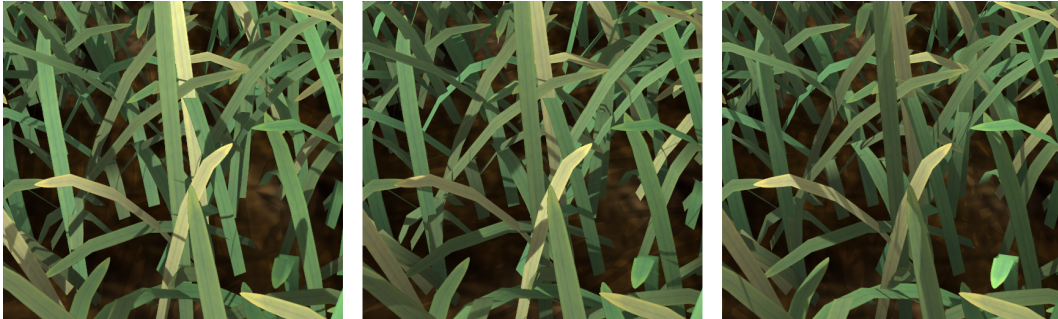
Figure 22: Results of dynamic lighting. A point light source is rotating around the grass surface. ( left ) Light source at the bottom of the image. ( middle ) Light source on the left. ( right ) Light source at the top of the image.
