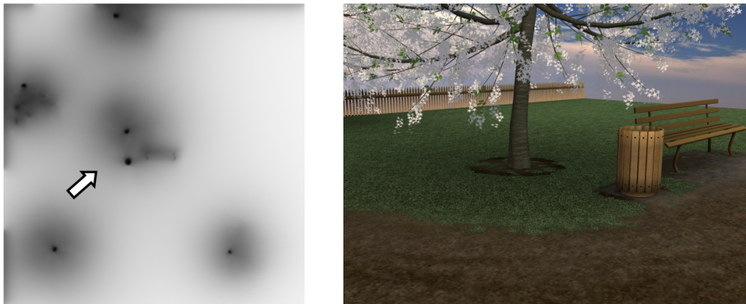
Figure 18: Ambient occlusion map covering the terrain and example of rendering. The arrow represents the camera position to get the image on the right.
