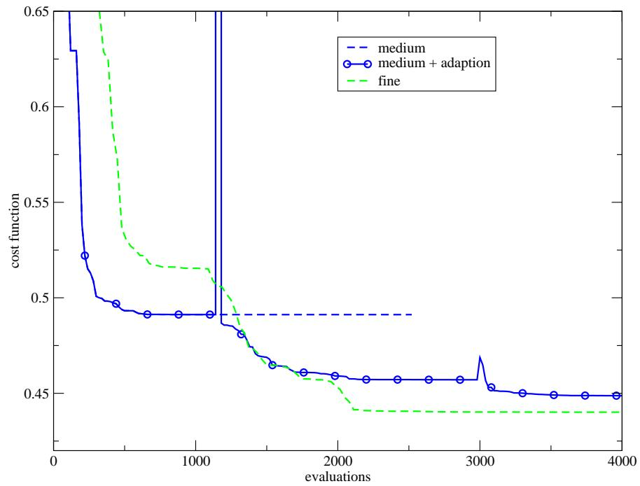
Figure 19: History of the cost function w.r.t. the number of evaluations : medium parameterization using the MSA method, with and without adaption.
