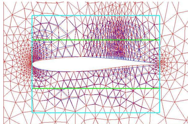
Figure 9: Example of FFD (cian) and blending (green) lattices.
