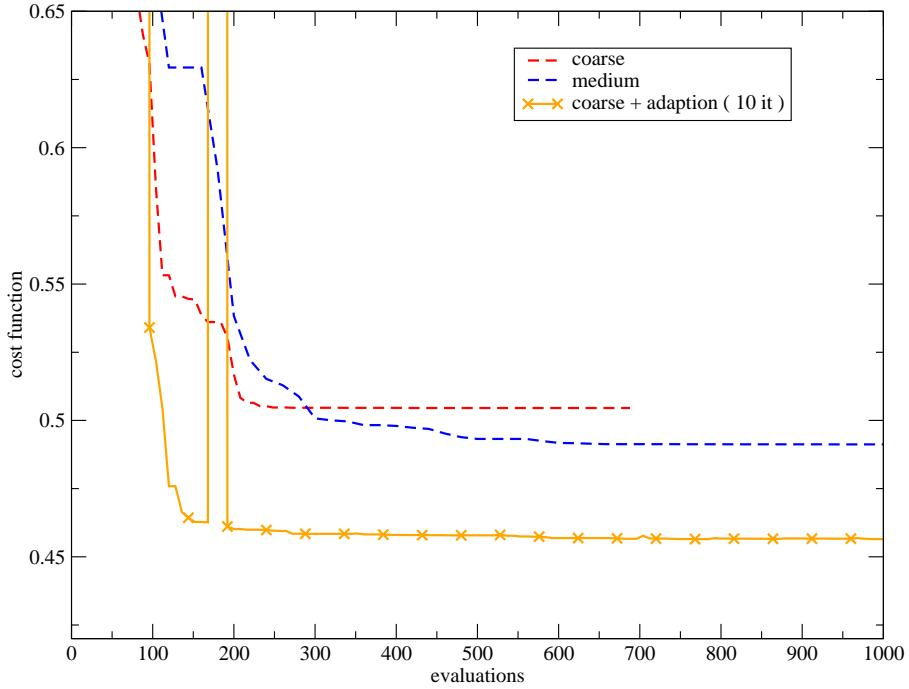
Figure 24: History of the cost function w.r.t. the number of evaluations : coarse parameterization using the MSA method, with and without progressive adaption (every 10 iterations).
