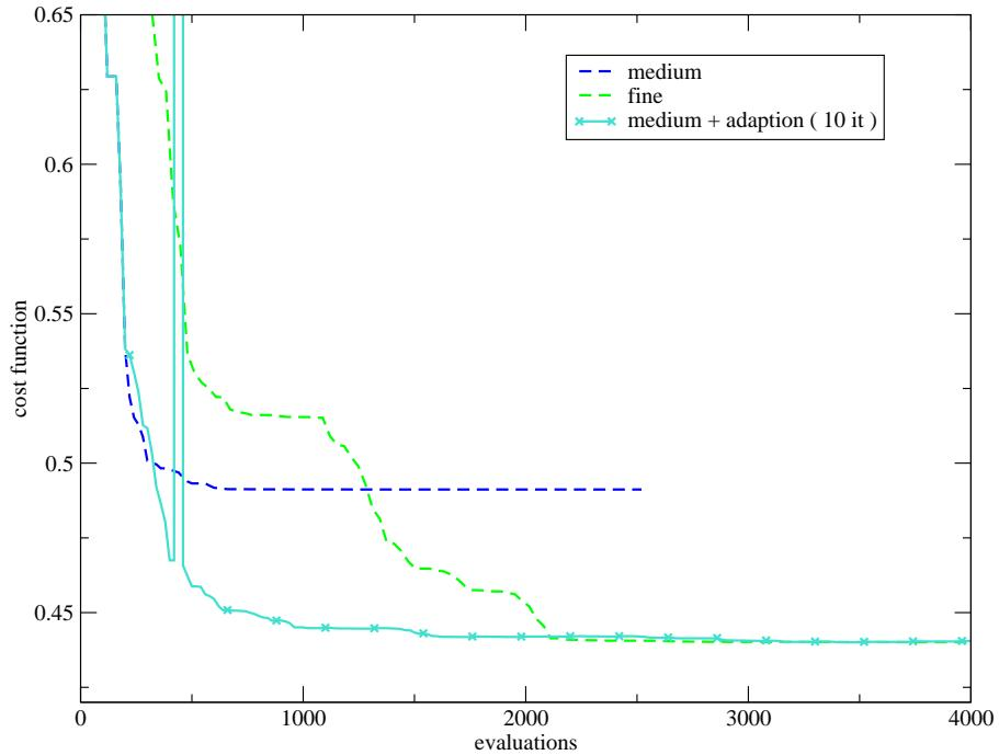
Figure 26: History of the cost function w.r.t. the number of evaluations : medium parameterization using the MSA method, with and without progressive adaption (every 10 iterations).
