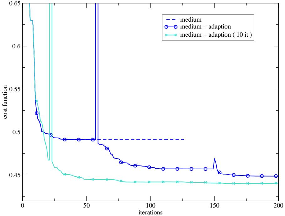
Figure 25: History of the cost function : medium parameterization using the MSA method, with and without progressive adaption (every 10 iterations).
