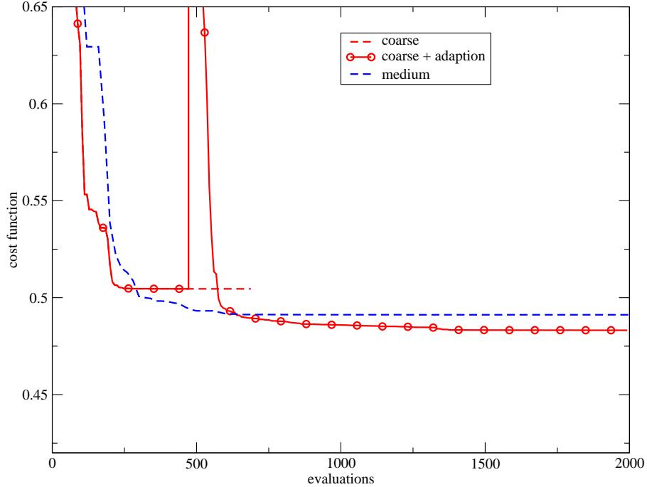
Figure 17: History of the cost function w.r.t. the number of evaluations : coarse parameterization using the MSA method, with and without adaption.
