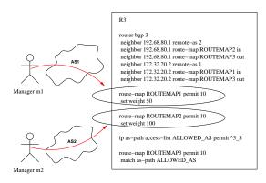
Figure 3: Network Sample CLI configuration
