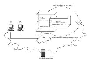
Figure 5: Conceptual security components
