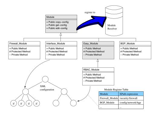
Figure 18: Module inheritance in YencaP
