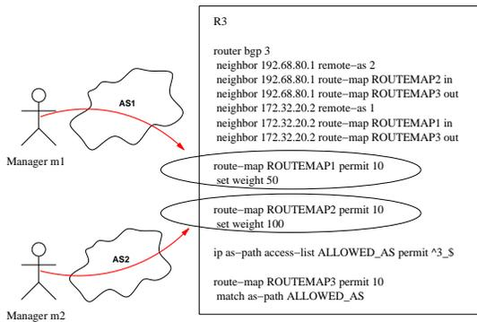
Figure 3: Network Sample CLI configuration
