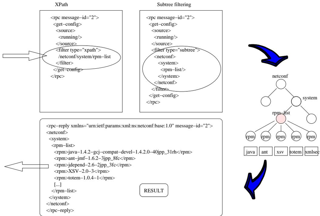
Figure 1: Simple get-config examples for RPM list retrieval
