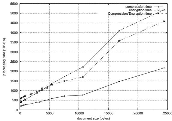
Figure 14: CPU time consumption with different combinations
