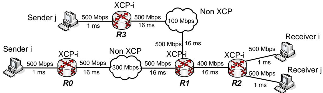
Figure 7: 2 upstream non-XCP queues,  $\Sigma input\_capacity = output\_capacity$
