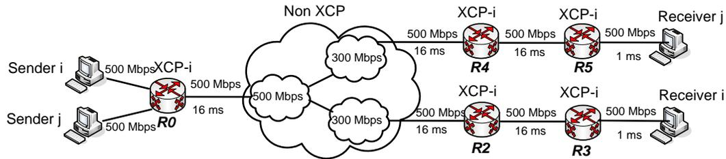
Figure 11: 1 non-XCP queue shared by XCP-capable downstream nodes
