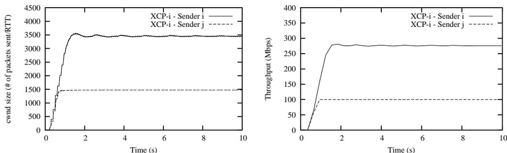
Figure 8: *cwnd* and throughput in the merge scenario
