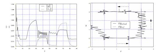
Figure 16: Estimates (57), pan control of the camera,  $\hat{c}_r = 0$
