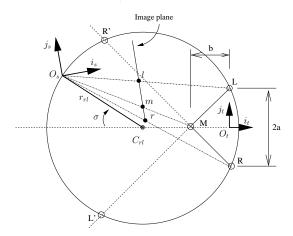
Figure 22: Camera pose reconstruction
