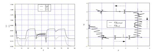
Figure 8: Nonlinear estimation of g: estimation of  $\varphi$  and inversion of  $\hat{\varphi}$ , pan-control,  $\hat{c}_r=0$
