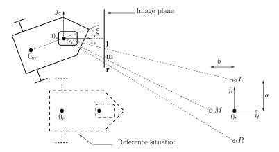
Figure 2: Unicycle-like robot with a vision-based sensor
