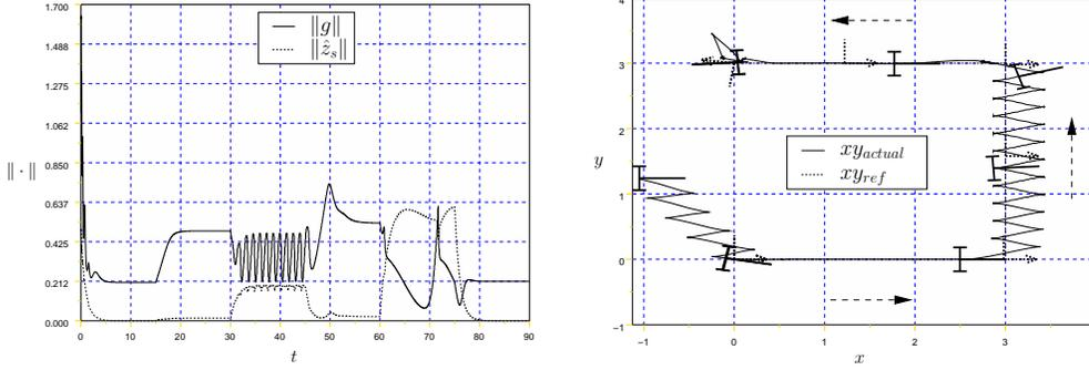
Figure 17: Estimates (58), pan-control of the camera,  $\hat{c}_r = 0$
