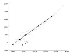
Figure 3: Bootstrap particle filter (BPF) with artificial Gaussian noise on (13): 0.025 m/s standard deviation on the velocity components and 25m on the position components.
