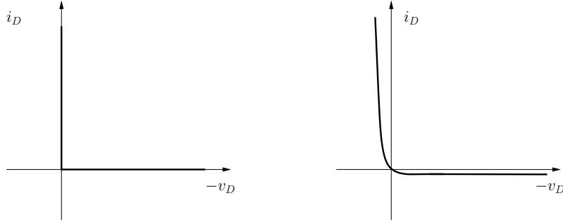
Figure 4.1: Non-smooth and smooth characteristics of a diode
