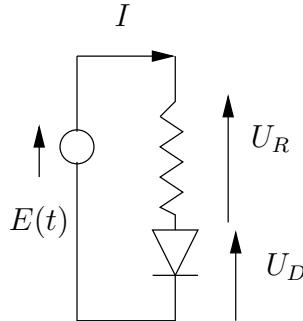
Figure 2.3: Polarization of a diode
