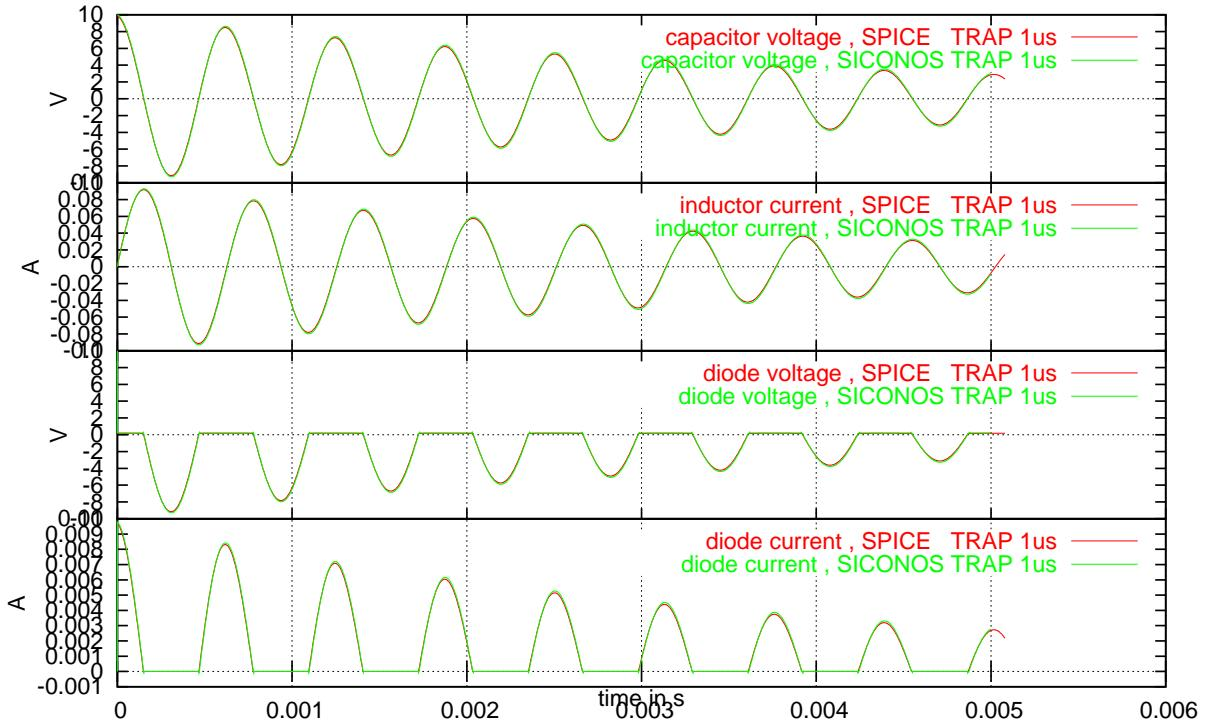
Figure 4.3: SPICE and SICONOS simulation results of RLCD circuit,  $1 \mu\text{s}$  time step
