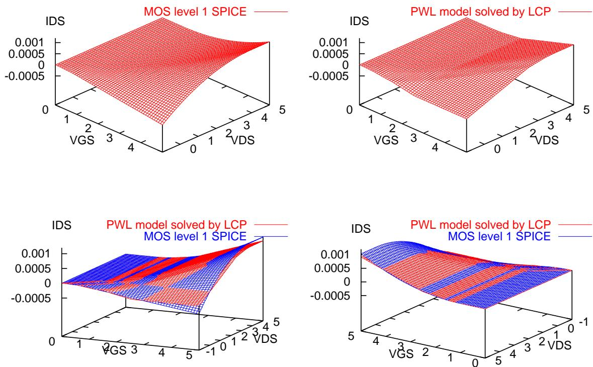
Figure 4.11: Static characteristic of an NMOS transistor with a simple PWL model and SPICE level 1 model
