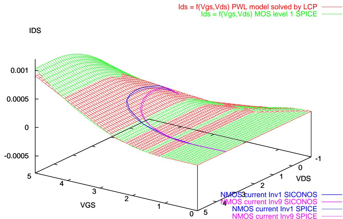
Figure 4.15: Plot of  $(V_{GS}, V_{DS}, I_{DS})$  values for inverters 1 and 9 and NMOS characteristics (perspective view)
