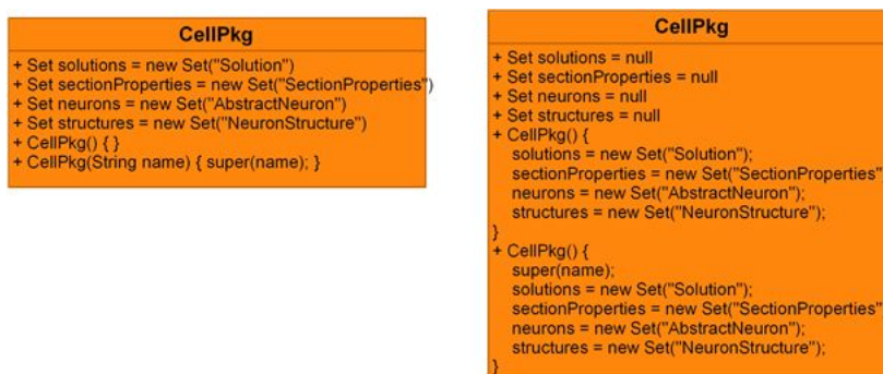
Figure 4: Initialization of attributes in the default constructors. Open arrows indicate inheritance, pointing from inheritors to their parents.
