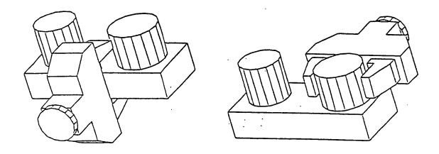
Figure 12: Two grasping positions computed by the system.
