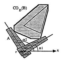
Figure 4: Computing the valid ranges of orientation associated to a translating and rotating polygonal object. (a) Determination of the set  $CO_D(B)$ . (b) Determination of the valid ranges of orientation of A relatively to  $CO_D(B)$ :  $[0 \ \alpha_1] \cup [\alpha_2 \ 2\pi]$ .
