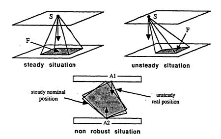
Figure 8: Stability and robustness properties. (a) Stable couple (S, F):  $proj(S) \in F$ . (b) Unstable couple (S, F):  $proj(S) \notin F$ . (c) Non robust couple  $(A_1, A_2)$ :  $proj(A_1) = proj(A_2) = straightline$ .
