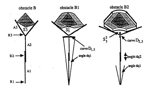
Figure 6: Propagating the position constraints along the arm.
