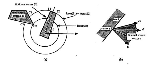
Figure 1: Computation of the contacts associated to a rotating object. (a) Potential contacts in a 2D exemple:  $(s_1, c_1)$ ,  $(s_2, c_2)$ ,  $(s'_1, c_2)$ . (b) Contact (s, f) locally valid:  $a_1 \cdot n \ge 0$  and  $a_2 \cdot n \ge 0$  and  $a_3 \cdot n \ge 0$ .
