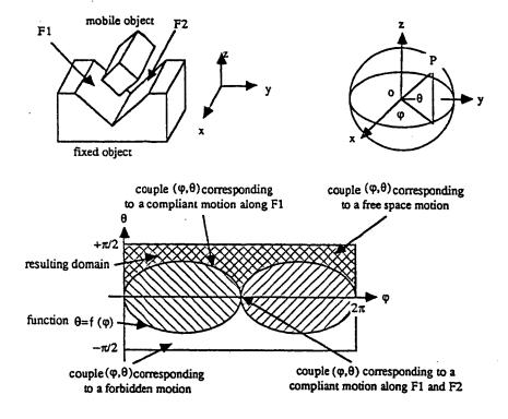
Figure 9: Representing the potential motions associated to a couple of planar contacts.
