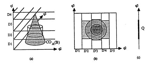
Figure 5: Computing an approximation of  $CO_A(B)$  for a three joints robot A. (a) Constructing the slices associated to  $q_1$ . (b) Representing the approximation of  $CO_A^{D_2}(B)$  associated with the slice  $D_2$ . (c) Representing the approximation of  $CO_A^{D_2 \times D_4'}(B)$  associated with the slices  $D_2$  and  $D_4'$ .
