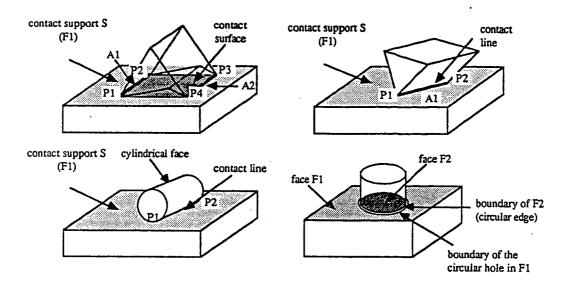
Figure 7: Example of some contacts: (a) Planar contact generated by a planar face and two edges. (b) Linear contact generated by a planar face and an edge. (c) Linear contact generated by a planar face and a cylindrical face. (d) Adjacent contact generated by two circular edges.
