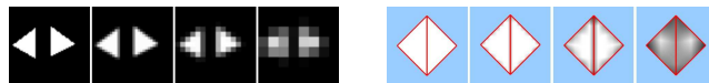
Figure 3: Left : four MIP-map levels of a texture atlas containing two regions. Right : The two regions are mapped on two adjacent triangles ( red ). One can see that texture background color bleeds at the edges.
