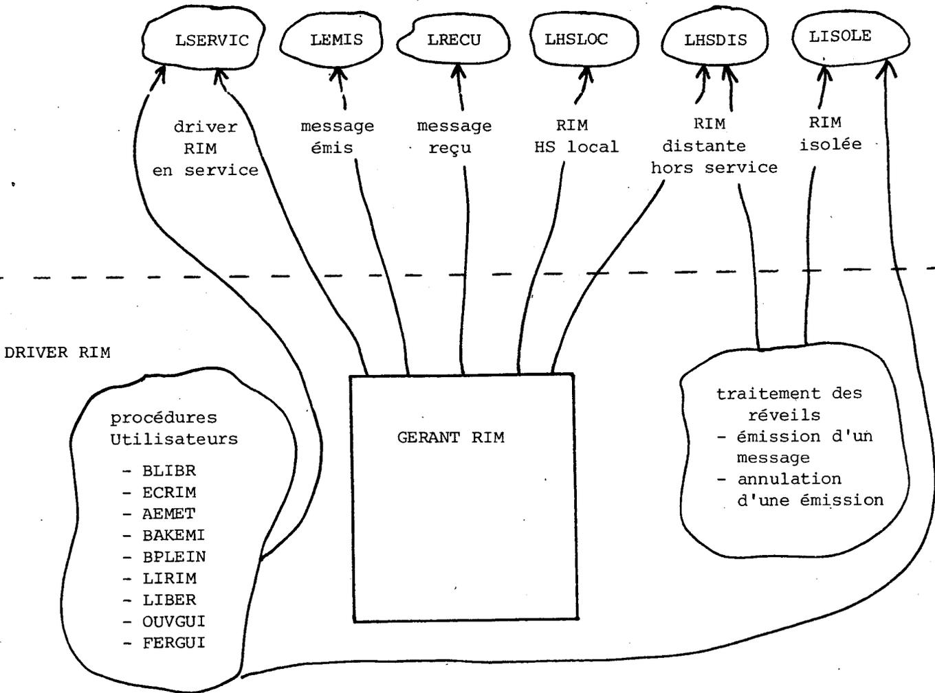
Figure V.21. - Structuration du driver RIM.
