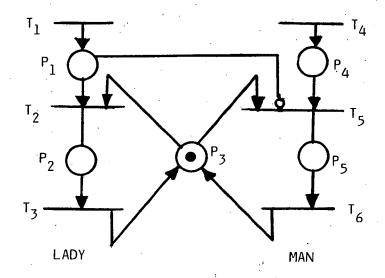
We could have eliminated the inhibitor arc by assigning priorities to transitions and by giving transition T2 a higher priority than transition T5 .
