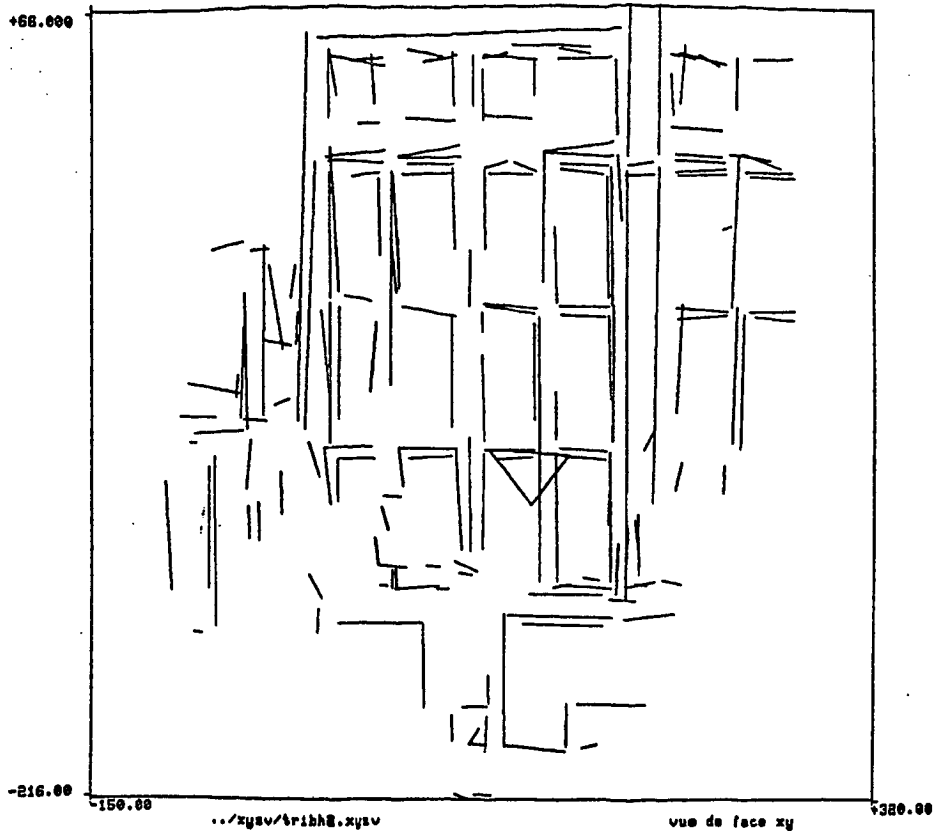
Figure 17: Horizontal and vertical projection of the reconstructed segments of the office room observed in position 2
