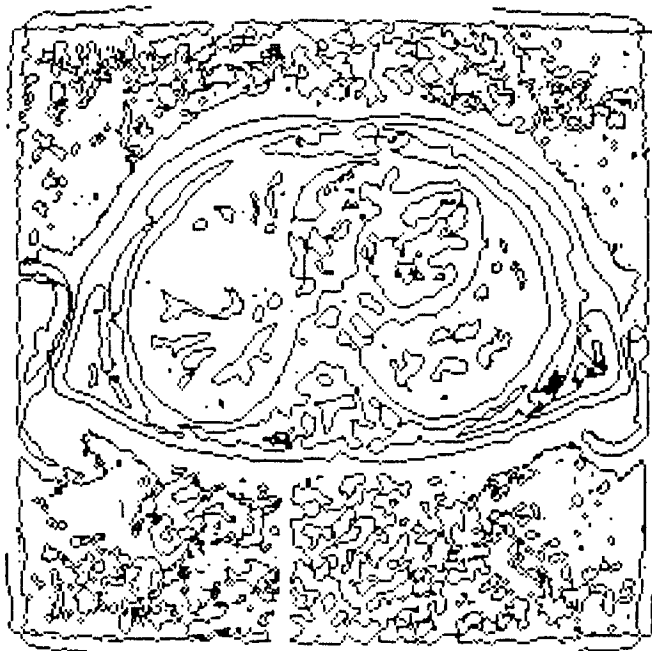
Figure 22 : 3d zero crossing without thresholding, Deriche filter, \alpha = 0.6
