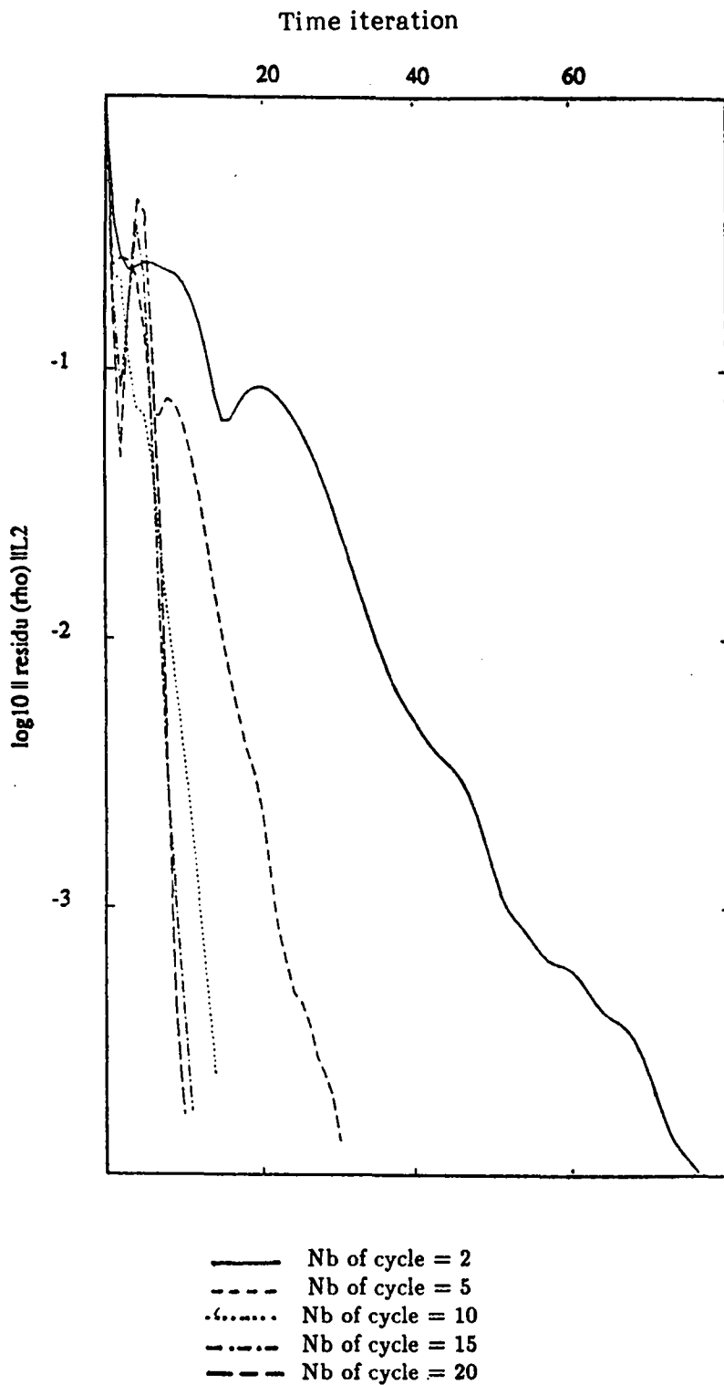
Figure 16 : Channel with bump ; Mach = .85 First-order spatial approximation Linear phase with Jacobi- 4-grid iteration, \omega = 1 Non linear time convergence with CFL = 1000 (comparison of various number of cycles in linear phase.)
