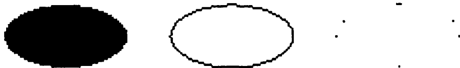
Figure 15: Results on a synthetic 2D ellipse : On left original image of the ellipse, on middle edges extracted and on left curvature extrema; The parameters of the filters are : \alpha = 1.5 for the smooth component, \alpha = 1.2 for the first derivatives, \alpha = 1.0 for the second derivatives and \alpha = 0.8 for the third derivatives. The two false curvature extrema could be removed by a simple thresholding using the maximum curvature
