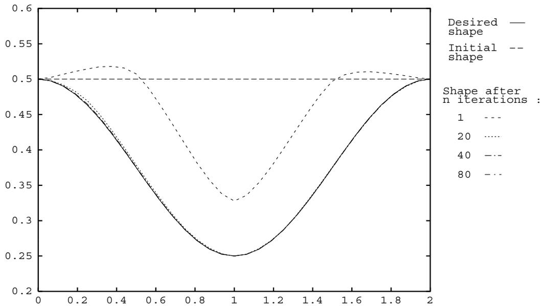
Figure 14: Successives shapes : Full V-cycle, nested cubic interpolation
