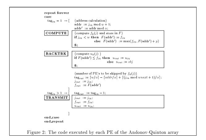
is shown in Fig 2 (it includes the book-keeping required for the backtracking part of the algorithm).
