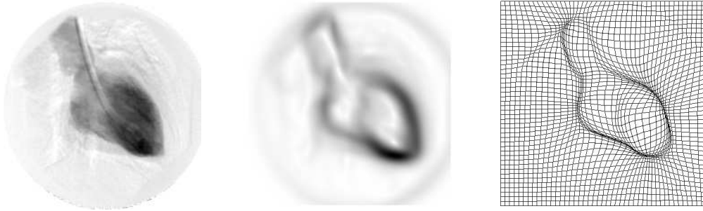
Figure 3: Adaptive deformation of a mesh. On left, raw image. On middle, gradient norm of the image function from which the mesh is deformed. On right, adaptive mesh. We started with a regular mesh having one node each four pixels. The density of nodes is increased near contour points.
