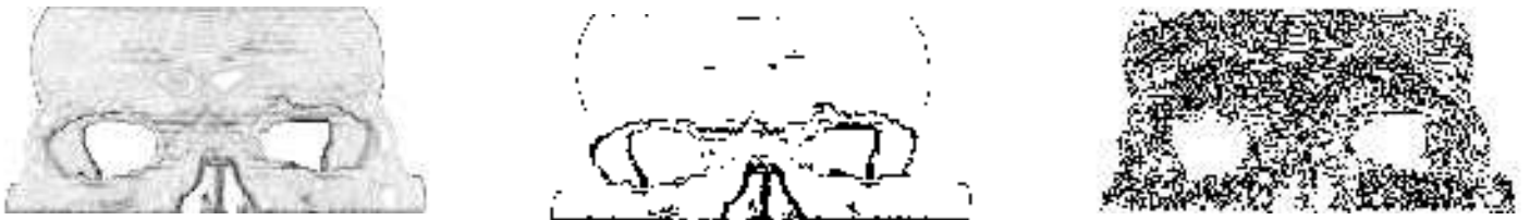
Figure 12: From left to right perspective views of : the maximum curvature, the high maximum curvature points, the zero-crossings of the extremality criterion : cross sections corresponding to position A; \sigma is set to 1 ; for this figure and the two following ones we only show the upper part of the skull.
