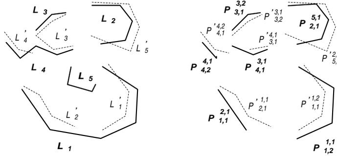
Figure 3: The registration algorithm has to find the portions  $P_{i,k}^{j,l}$  and  $P_{j,l}^{i,k}$ , respectively the  $k^{\text{th}}$  portion of  $L_i$  which corresponds to the  $l^{\text{th}}$  portion of  $L_j$  and vice versa.
