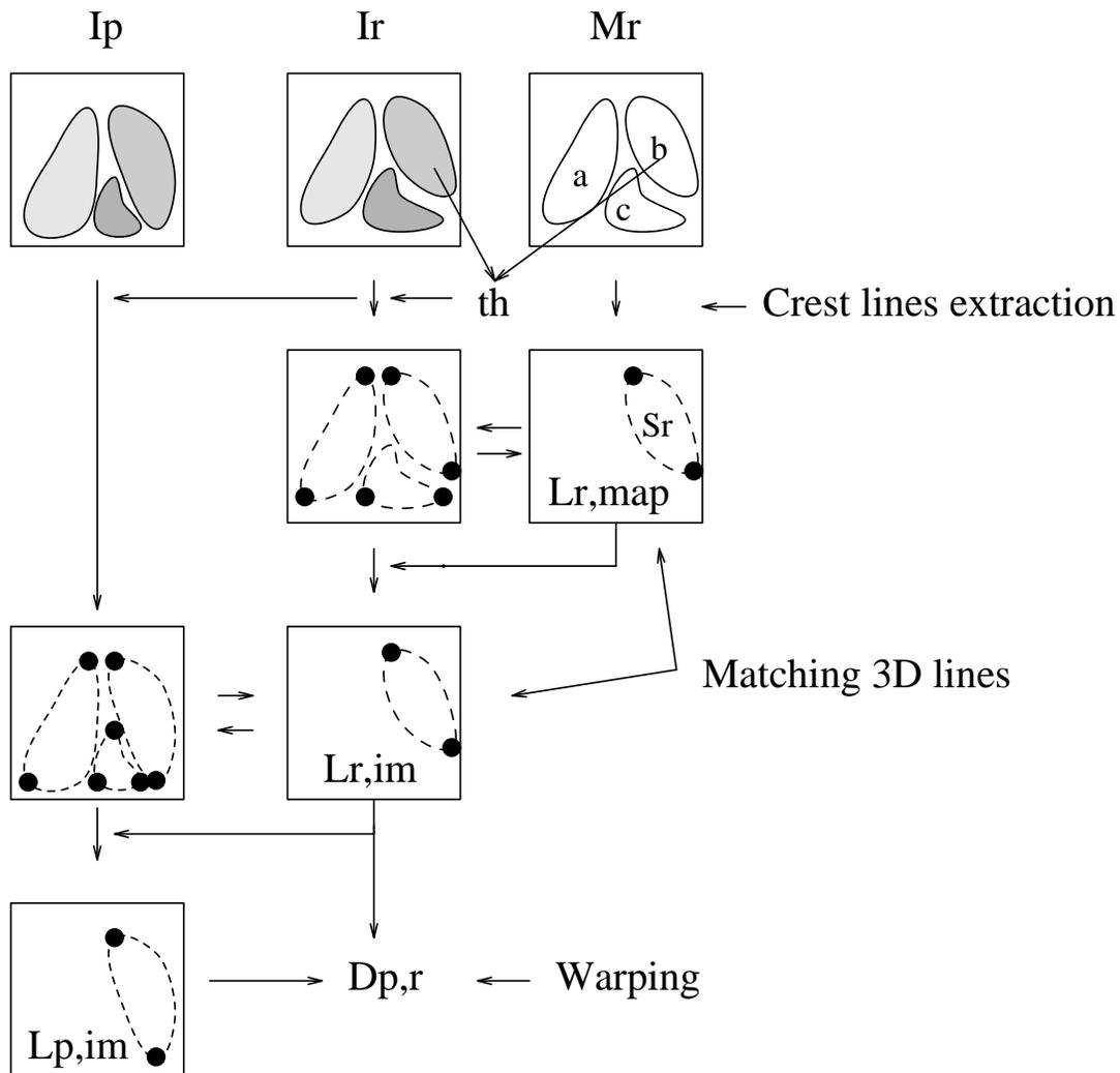
Figure 1: Crest lines  $L_{r,map}$  are extracted from the reference map and used to find the corresponding lines  $L_{r,im}$  in the reference image  $I_r$ . The crest lines  $L_{p,im}$  are extracted from the new image  $I_p$ , using  $L_{r,im}$ . This gives a set of correspondence and warping is applied to obtain the final deformation  $D_{p,r}$ .
