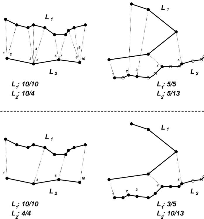
Figure 4: *The topological constraints help to remove inconsistent couples of linked points: left, some points have too many correspondents, right, a part of  $L_1$  have a erroneous correspondent on  $L_2$ .*
