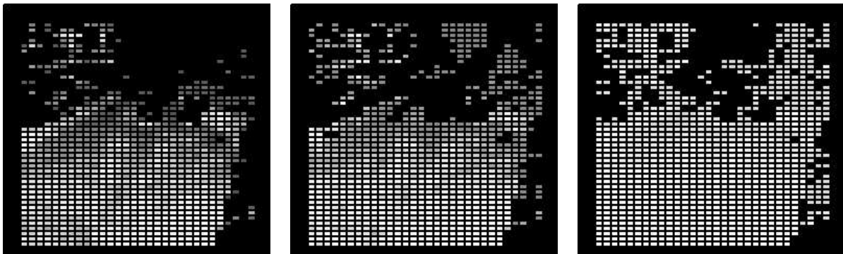
Figure 13: Traversability map from the distribution of slopes on real data. Left: small admissible region \theta = 20^\circ ; Center: medium admissible region \theta = 45^\circ ; Right: large admissible region \theta = 75^\circ .
