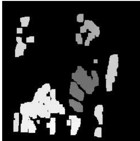
Figure 16: The disparity map obtained from the rectified images of Figure 15.
