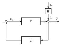
Figure 10: LQG disturbance rejection loop
