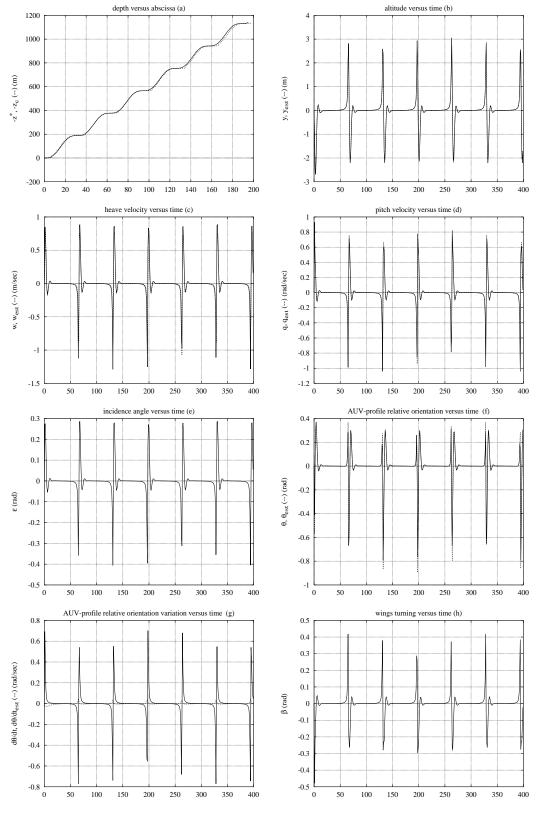
Figure 23: Simulation on "quasi" sinusoidal bottom profile using the LQG/LTR+EKF controller. Main parameters value: bottom period:  $\approx 70sec$ , vehicle initial orientation=0rad, Rc=30.0, Ro=0.1, Ad=-.1, Cd=-Ad, Gd=5.0. Advancement velocity:  $u_0 = 3m/sec$
