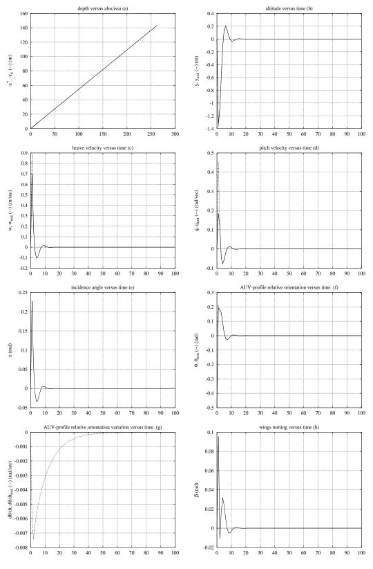
Figure 19: Simulation on linear bottom profile using the LQG/LTR+EKF controller. Main parameters value: bottom slope=0.5rad, vehicle initial orientation=0rad, Rc=30.0, Ro=0.1, Ad=-.1, Cd=-Ad, Gd=5.0. Advancement velocity:  $u_0=3m/sec$
