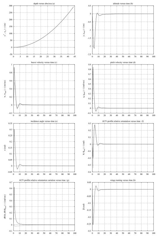
Figure 21: Simulation on parabolic bottom profile using the LQG/LTR+EKF controller. Main parameters value: bottom:  $z^* = -0.15x^{*^2} + z0$ , vehicle initial orientation=0rad, Rc=30.0, Ro=0.1, Ad=-.1, Cd=-Ad, Gd=5.0. Advancement velocity:  $u_0 = 3m/sec$
