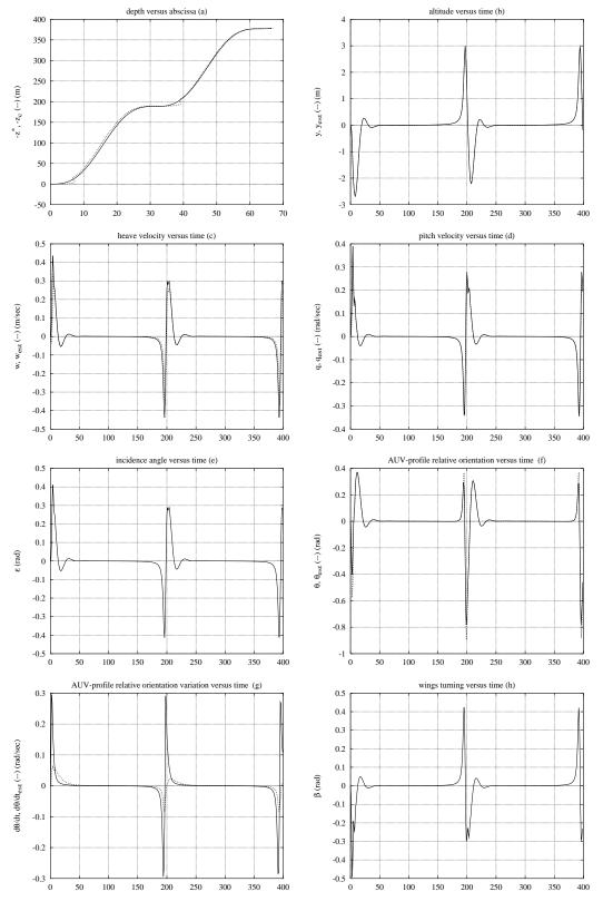
Figure 17: Simulation on "quasi" sinusoidal bottom profile using the LQG/LTR+EKF controller. Main parameters value: bottom period:  $\approx 210sec$ , vehicle initial orientation=0rad, Rc=30.0, Ro=0.1, Ad=-.1, Cd=-Ad, Gd=5.0. Advancement velocity:  $u_0=1m/sec$
