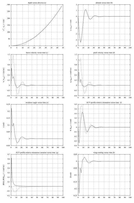
Figure 20: Simulation on parabolic bottom profile using the LQG/LTR controller. Main parameters value : bottom :  $z^* = -0.15x^{*^2} + z0$ , vehicle initial orientation=0rad, Rc=30.0, Ro=0.1, Ad=-.1, Cd=-Ad, Gd=5.0. Advancement velocity :  $u_0 = 3m/sec$
