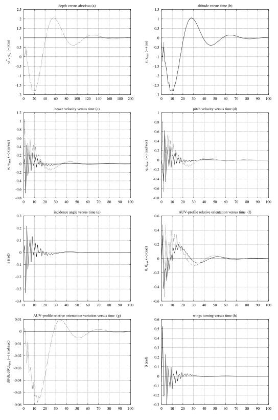
Figure 28: Simulation on linear bottom profile using the LQG/LTR linear controller. Main parameters value: bottom slope=0.5rad, vehicle initial orientation=0rad, Rc=100.0, Ro=1.0, Ad=-.1, Cd=-Ad, Gd=5.0. Advancement velocity:  $u_0 = 2m/sec$
