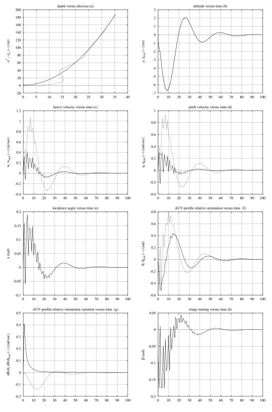
Figure 26: Simulation on parabolic bottom profile using the LQG/LTR controller. Main parameters value : bottom :  $z^* = -0.15x^{*^2} + z0$ , vehicle initial orientation=0rad, Rc=50.0, Ro=1.0, Ad=-.1, Cd=-Ad, Gd=5.0. Advancement velocity :  $u_0 = 2m/sec$
