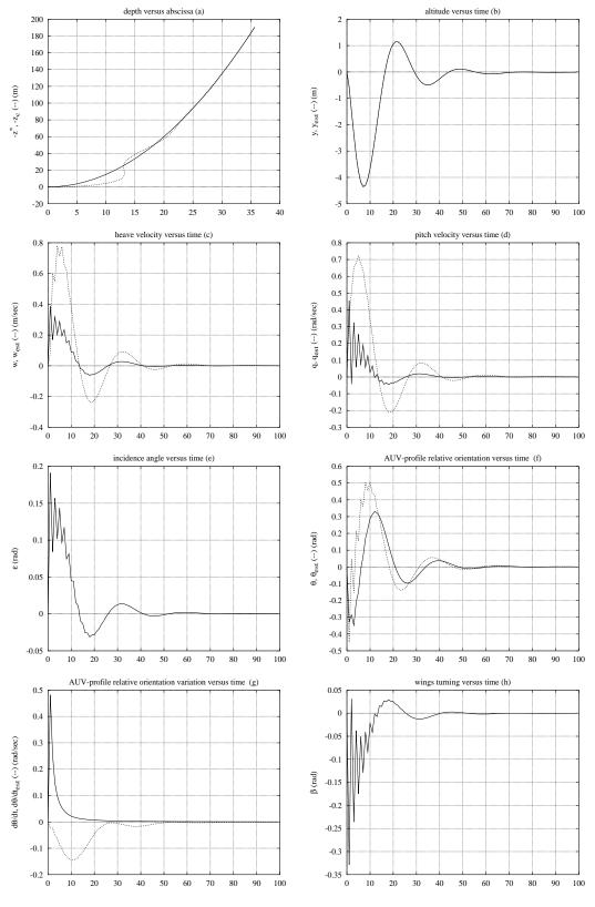
Figure 4: Simulation on parabolic bottom profile using the LQG/LTR controller. Main parameters value: bottom:  $z^* = -0.15x^{*2} + z0$ , vehicle initial orientation=0rad, Rc=30.0, Ro=0.1, Ad=-.1, Cd=-Ad, Gd=5.0
