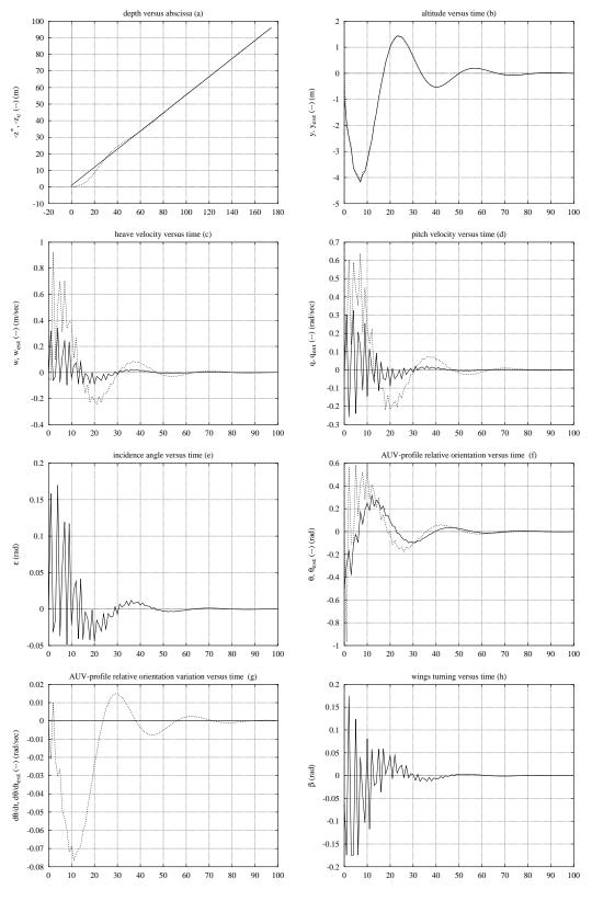
Figure 24: Simulation on linear bottom profile using the LQG/LTR linear controller. Main parameters value: bottom slope=0.5rad, vehicle initial orientation=0rad, Rc=50.0, Ro=1.0, Ad=-.1, Cd=-Ad, Gd=5.0. Advancement velocity:  $u_0 = 2m/sec$
