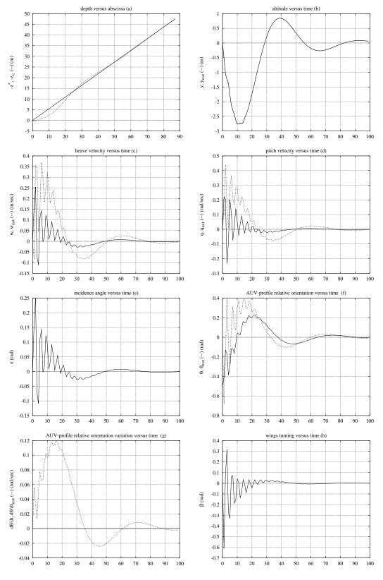
Figure 12: Simulation on linear bottom profile using the LQG/LTR linear controller. Main parameters value: bottom slope=0.5rad, vehicle initial orientation=0rad, Rc=30.0, Ro=0.1, Ad=-.1, Cd=-Ad, Gd=5.0. Advancement velocity:  $u_0 = 1m/sec$
