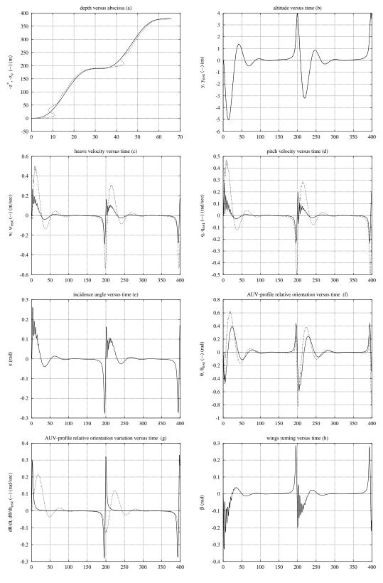
Figure 16: Simulation on "quasi" sinusoidal bottom profile using the LQG/LTR controller. Main parameters value: bottom period:  $\approx 210sec$ , vehicle initial orientation=0rad, Rc=30.0, Ro=0.1, Ad=-.1, Cd=-Ad, Gd=5.0. Advancement velocity:  $u_0=1m/sec$
