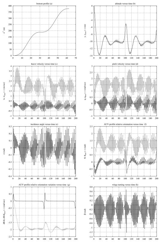
Figure 32: Simulation on "quasi" sinusoidal bottom profile using the LQG/LTR controller. Main parameters value : vehicle initial orientation=0rad, Rc=10.0, Ro=1.0, Ad=-.1, Cd=-Ad, Gd=5.0. Advancement velocity :  $u_0=2m/sec$
