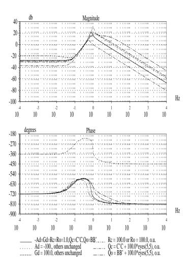
Figure 2: Magnitude frequency responses for LQG/LTR controller with various parameters values.
