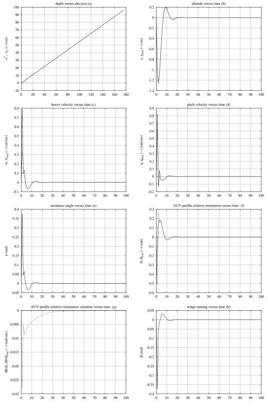
Figure 7: Simulation on linear bottom profile using the LQG/LTR+EKF controller. Main parameters value: bottom slope=0.5rad, vehicle initial orientation=0rad, Rc=30.0, Ro=0.1, Ad=-.1, Cd=-Ad, Gd=5.0 (identical to those for simulations using LQG/LTR controller before)
