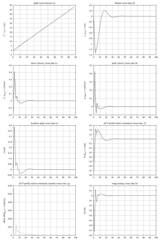
Figure 13: Simulation on linear bottom profile using the LQG/LTR+EKF controller. Main parameters value: bottom slope=0.5rad, vehicle initial orientation=0rad, Rc=30.0, Ro=0.1, Ad=-.1, Cd=-Ad, Gd=5.0. Advancement velocity:  $u_0=1m/sec$
