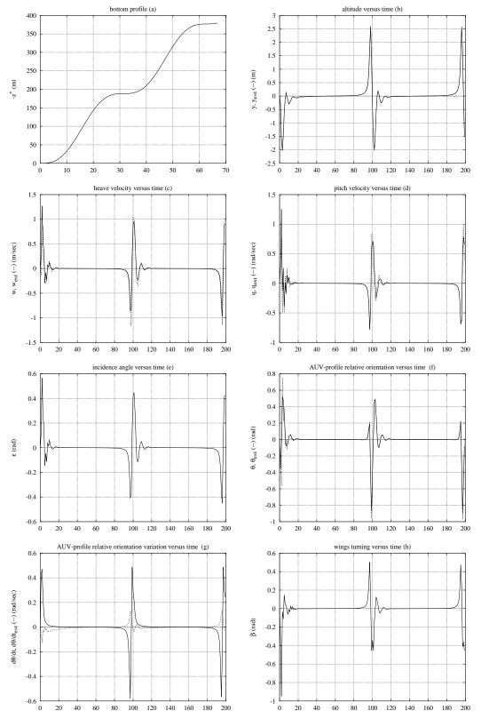
Figure 33: Simulation on "quasi" sinusoidal bottom profile using the LQG/LTR+EKF controller. Main parameters value: vehicle initial orientation=0rad, Rc=10.0, Ro=1.0, Ad=-.1, Cd=-Ad, Gd=5.0. Advancement velocity:  $u_0=2m/sec$
