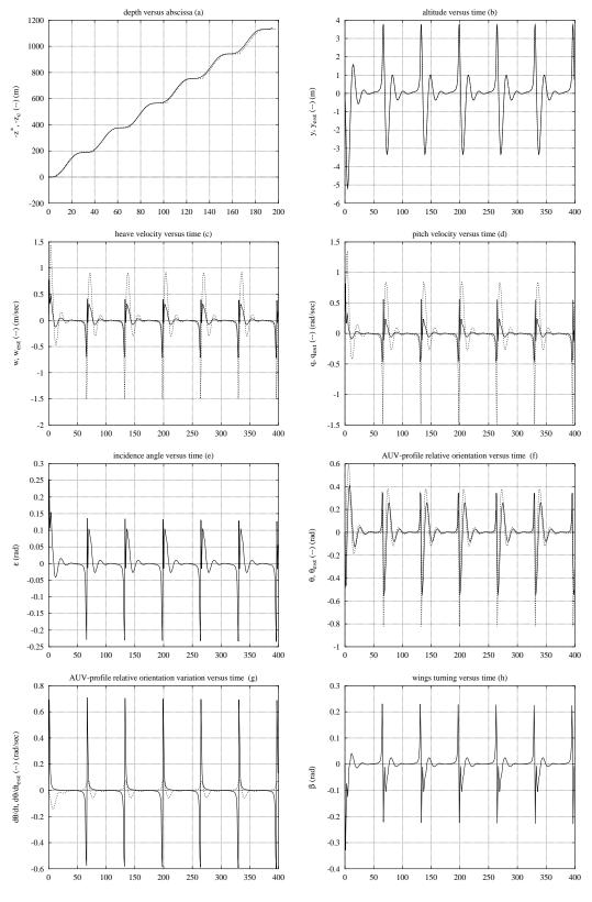
Figure 22: Simulation on "quasi" sinusoidal bottom profile using the LQG/LTR controller. Main parameters value : bottom period :  $\approx 70sec$ , vehicle initial orientation=0rad, Rc=30.0, Ro=0.1, Ad=-.1, Cd=-Ad, Gd=5.0. Advancement velocity :  $u_0=3m/sec$
