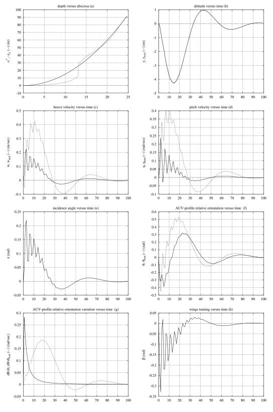
Figure 14: Simulation on parabolic bottom profile using the LQG/LTR controller. Main parameters value : bottom :  $z^* = -0.15x^{*^2} + z0$ , vehicle initial orientation=0rad, Rc=30.0, Ro=0.1, Ad=-.1, Cd=-Ad, Gd=5.0. Advancement velocity :  $u_0 = 1m/sec$
