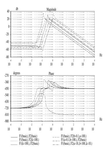
Figure 6: Magnitude frequency responses for frequency-weighted LQG controllers. The form of the filters is a first-order simple lead-lag network: F(s) = k(1+s/a)/(1+s/b). For the low-pass filter F1, the basic configuration has the following values: k=1.0, a=1.0, b=0.01. For the high-pass filter F2, the basic configuration has the following values: k=1.0, a=0.01, b=1.0.
