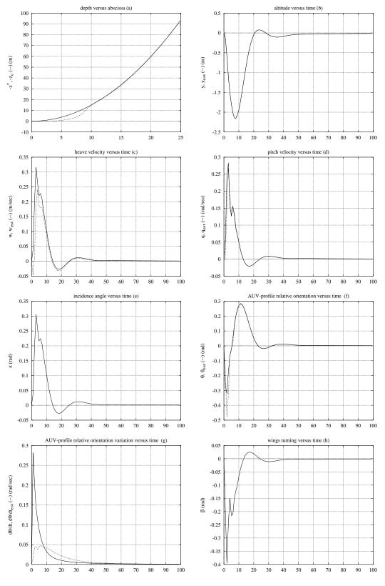
Figure 15: Simulation on parabolic bottom profile using the LQG/LTR+EKF controller. Main parameters value: bottom:  $z^* = -0.15x^{*^2} + z0$ , vehicle initial orientation=0rad, Rc=30.0, Ro=0.1, Ad=-.1, Cd=-Ad, Gd=5.0. Advancement velocity:  $u_0 = 1m/sec$
