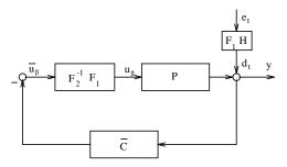
Figure 11: Frequency-weighted LQG disturbance rejection loop
