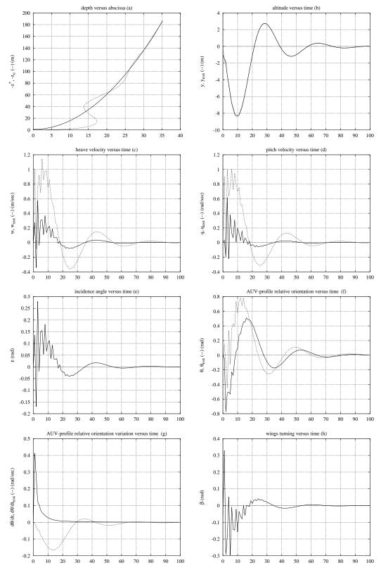
Figure 30: Simulation on parabolic bottom profile using the LQG/LTR controller. Main parameters value : bottom :  $z^* = -0.15x^{*^2} + z0$ , vehicle initial orientation=0rad, Rc=100.0, Ro=1.0, Ad=-.1, Cd=-Ad, Gd=5.0. Advancement velocity :  $u_0 = 2m/sec$
