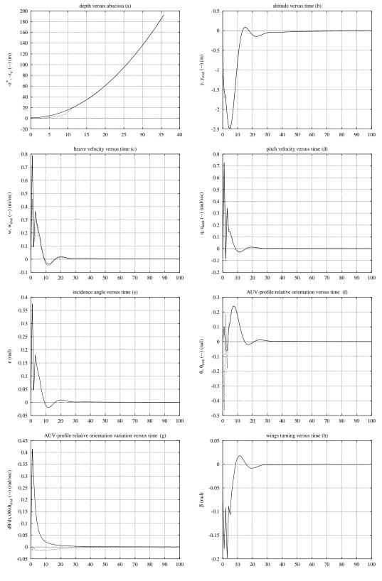
Figure 31: Simulation on parabolic bottom profile using the LQG/LTR+EKF controller. Main parameters value: bottom:  $z^* = -0.15x^{*2} + z0$ , vehicle initial orientation=0rad, Rc=100.0, Ro=1.0, Ad=-.1, Cd=-Ad, Gd=5.0. Advancement velocity:  $u_0 = 2m/sec$
