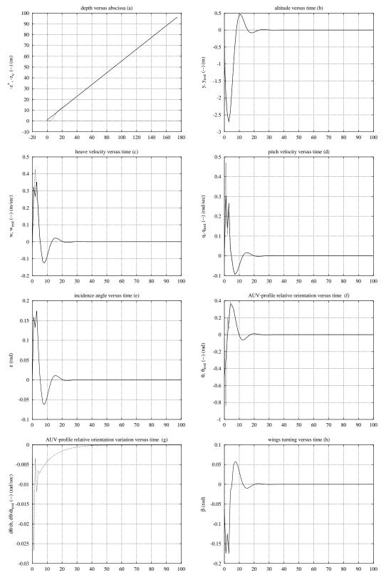
Figure 25: Simulation on linear bottom profile using the LQG/LTR+EKF controller. Main parameters value: bottom slope=0.5rad, vehicle initial orientation=0rad, Rc=50.0, Ro=1.0, Ad=-.1, Cd=-Ad, Gd=5.0. Advancement velocity:  $u_0 = 2m/sec$
