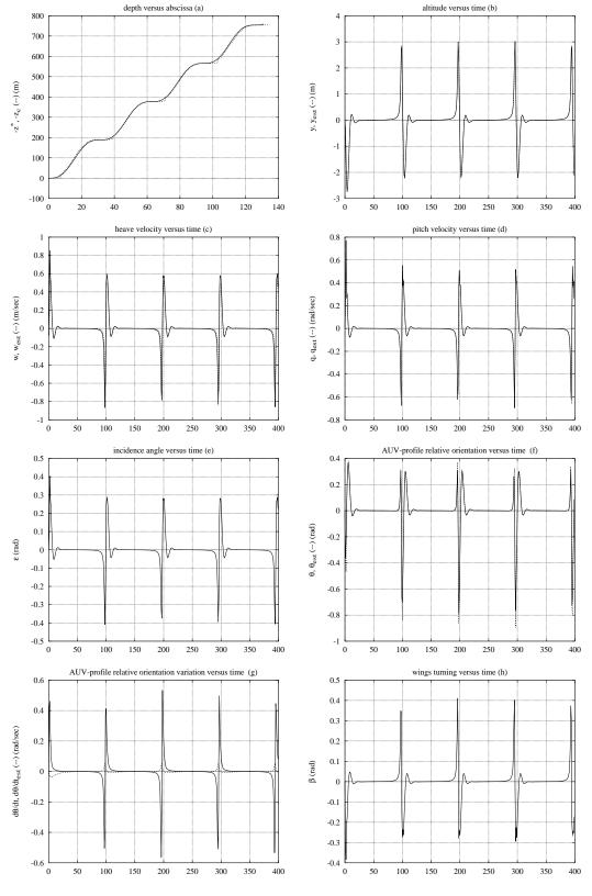
Figure 9: Simulation on "quasi" sinusoidal bottom profile using the LQG/LTR+EKF controller. Main parameters value: bottom period:  $\approx 100sec$ , vehicle initial orientation=0rad, Rc=30.0, Ro=0.1, Ad=-.1, Cd=-Ad, Gd=5.0 (identical to those for simulations using LQG/LTR controller before)
