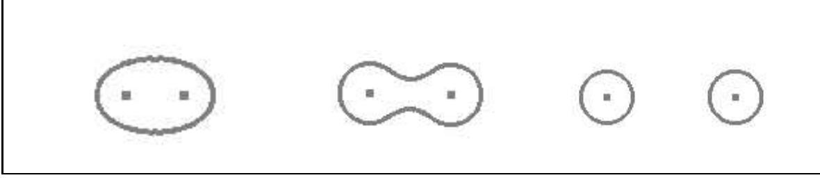
Figure 2: *Iso-contours obtained with two positive control points: given an iso-value, two positive control points and their radius of influence, the shape of the iso-contour changes continuously and finally can break itself into two connected components if the control points are too far away from each other.*
